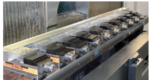
▲ On the 3 m linear table, 10 vises are mounted with the parallel specification.
