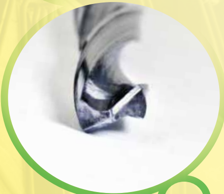
Tool with weared cutting edges
