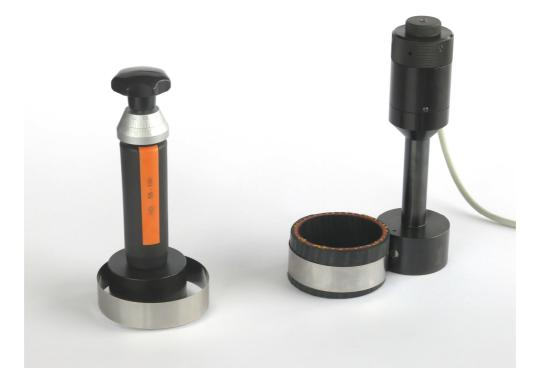
The Novometer<sup>®</sup> measuring instrument family has been complemented with a version for outside diameters. The overall diameter range is from 22 -330 mm and there is an analog design with a reading of 0,1 mm as well as a digital version with a reading of 0,01 mm.
