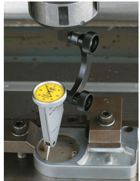
Centering of a bore
