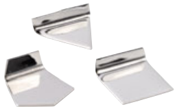
Milligram weights, flat polygonal sheet
