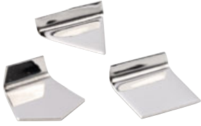
Milligram weights, flat polygonal sheet
