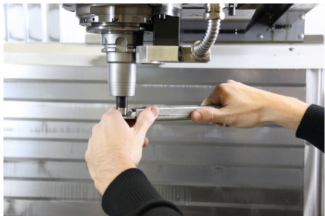
Important for the sensitive tuning is an additional placing of the hand on the exchange milling head. This means the torque can be better maintained.
