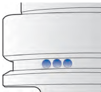
Fine-balanced with balancing bores in the flange
