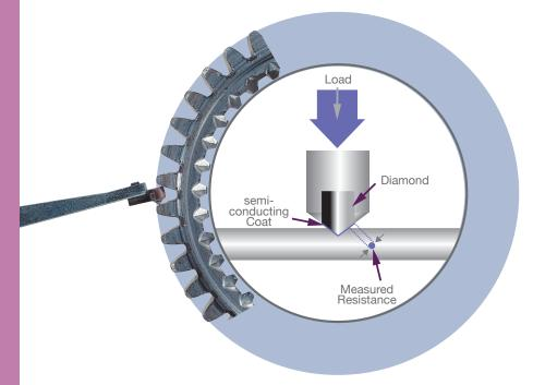
The diamond indenter can be compared to a little potentiometer, which, while gradually penetrating into the material, obtains all the data (load-hardness) during the whole phase of load application.
