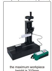
heavy duty test stand (optional)
