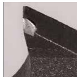
Damaged tooth, not run-in
