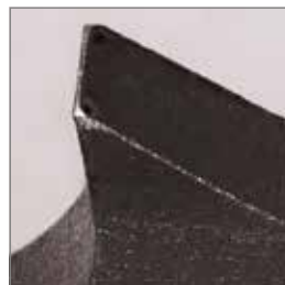
Damaged tooth, after running-in
