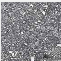
Structure image of the tooth tip material (M42 HSS)
