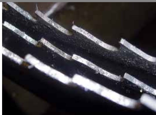
Chips sticking to the base of the tooth
