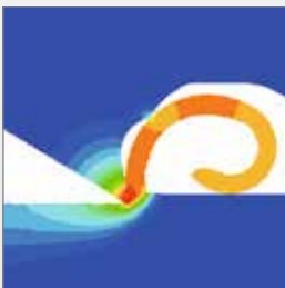
New tooth design with chip breaker
